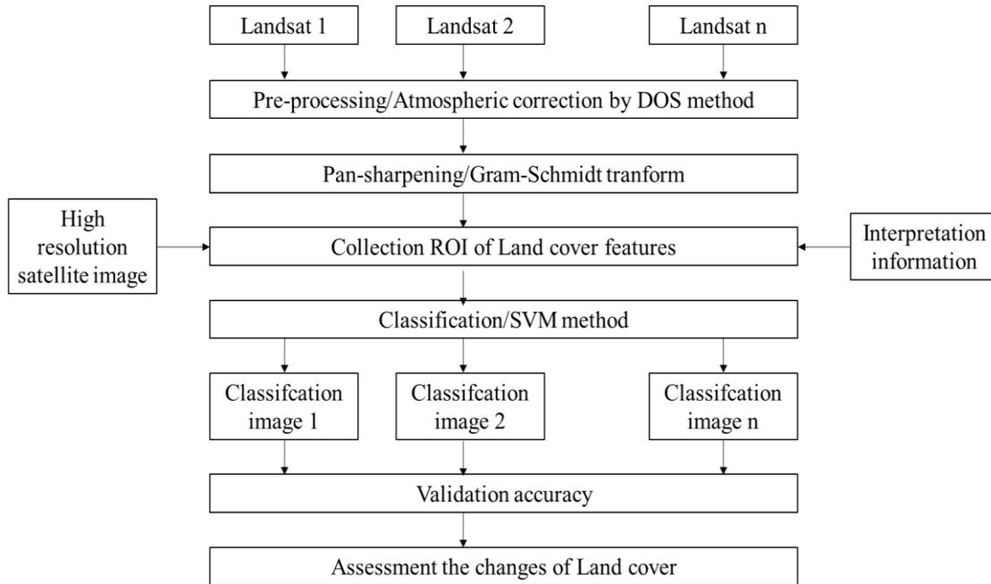
Figure 3. The workflow of the proposed method.
