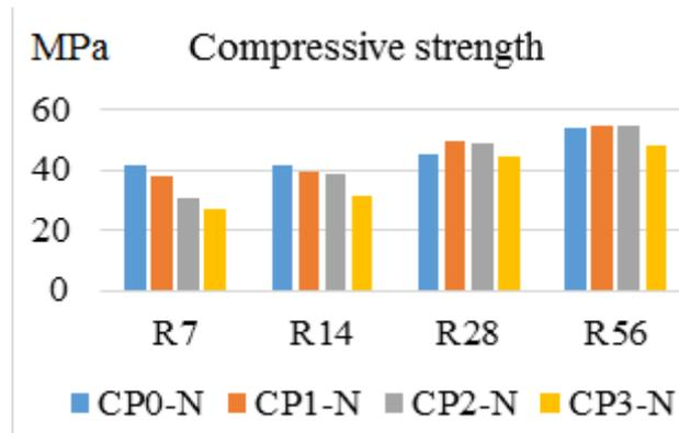
Figure 5. The development of compressive strength (using BASF 8588 additive).
