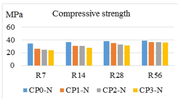
Figure 3. The development of compressive strength (using Sikament NN additives).
