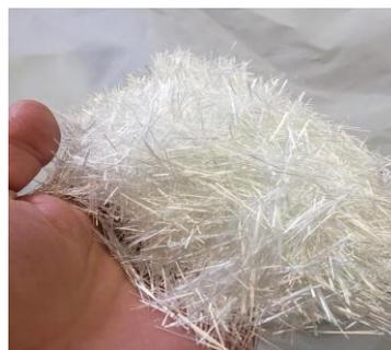
*Figure 2. Reinforced glass fiber.*
