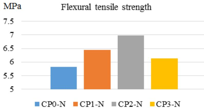
Figure 6. The development of Flexural tensile strength (using BASF 8588 additive).
